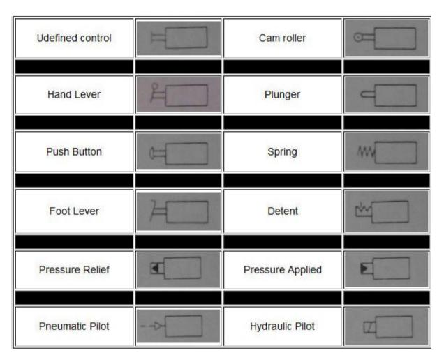
Figure 2 - Pneumatic Valve Control
