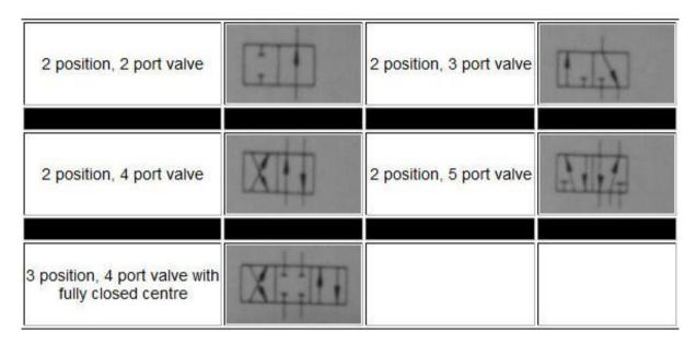
**Figure 3 - Directional Control Valves**
